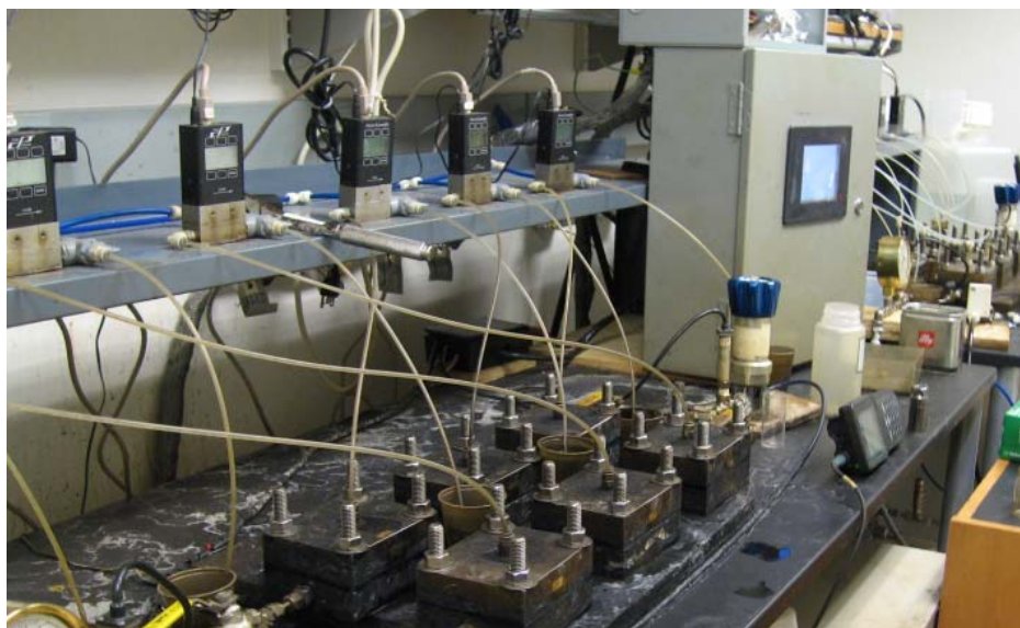
Figure 3: Flat-sheet Cell Testing Bench
