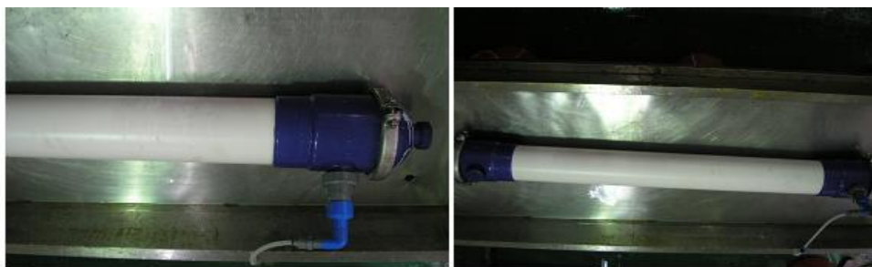
Figure 3: Membrane Module Leak Test
