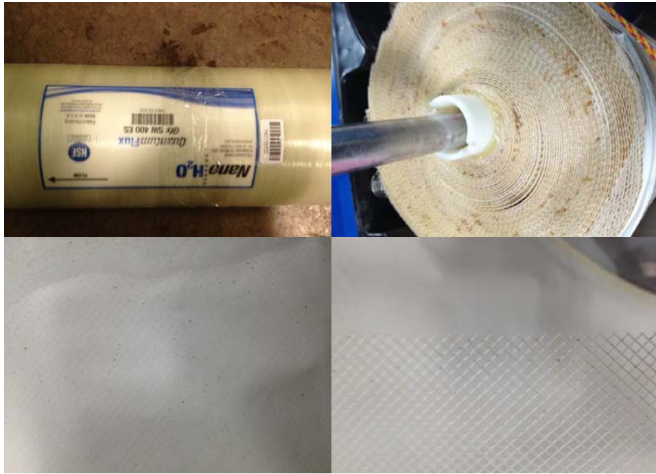
Figure 4. Lead Element Autopsy
