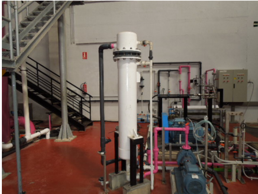
Figure 3: Pilot Test Pressure Vessel and Instrumentations
